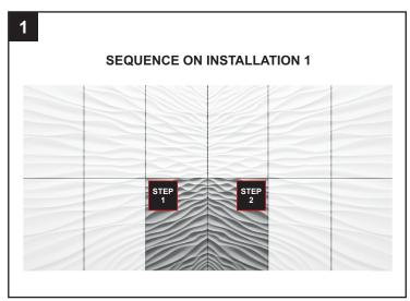
The sequence of unpacking and installing Illusion model. Open the box, take two first panels from the wooden box and mount them at the wall. Keeping recommended sequence, will guarantee the optimal effect of installation. Keep this sequence while installing at the wall.
